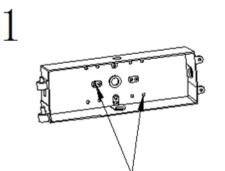
Using screws to install the power supply box onto the solid wall
