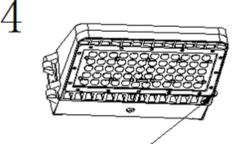
Close the body using screws and tighten them
