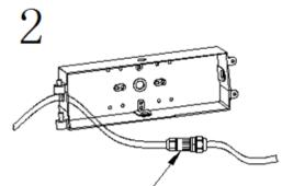
Open the wire-connecting box, connect the input wire of the LED driver with the AC input wire then close the box
